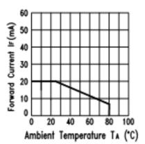
Fig.3 Forward Current Derating Curve
