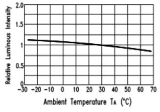
Fig.5 Luminous Intensity vs.Ambient Temperature
