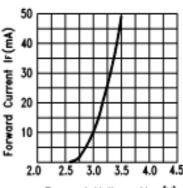
Forward Voltage Vr (V) Fig.2 Forward Current vs. Forward Voltage
