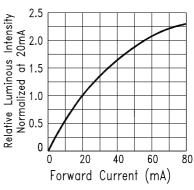
Fig.4 Relative Luminous Intensity vs. Forward Current
