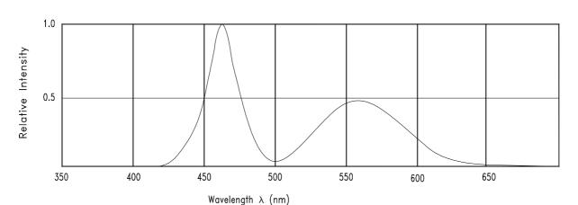
Fig.1 Relative Intensity vs. Wavelength
