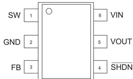
**600mA, 1.2MHz, Micropower Synchronous Step-Up Converter****Absolute Maximum Ratings<sup>1</sup>**
