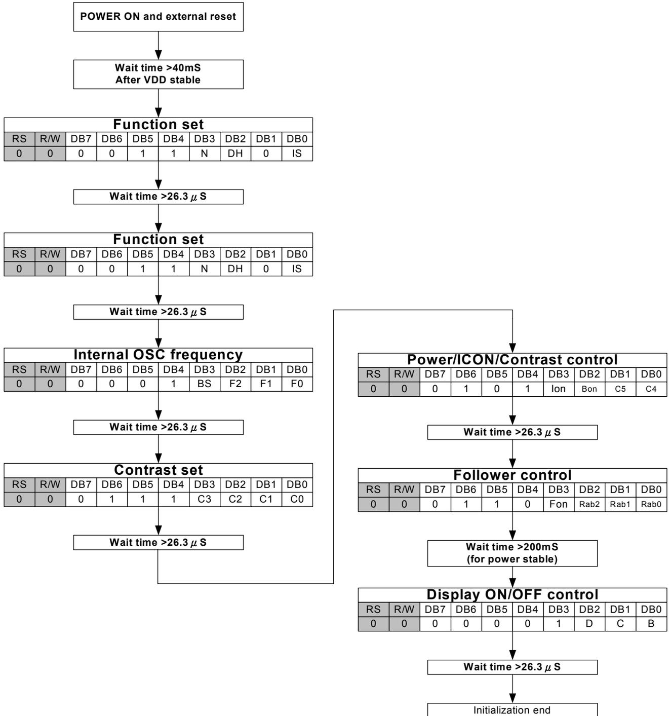
➤ **Initial Program Code Example For 8051 MPU(Serial Interface):**
