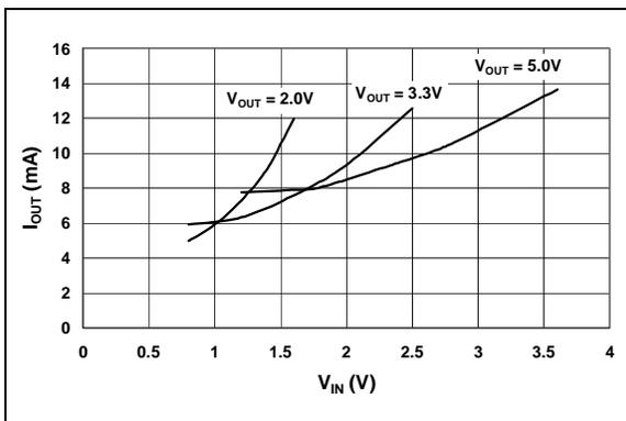
**FIGURE 2-15:** PFM / PWM Threshold Current vs.  $V_{IN}$ .
