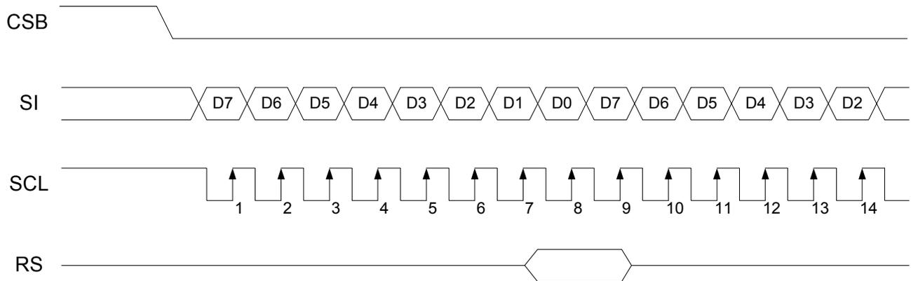
**Note:**The falling edge must cause on CSB before the serial clock ( SCL ) active.
