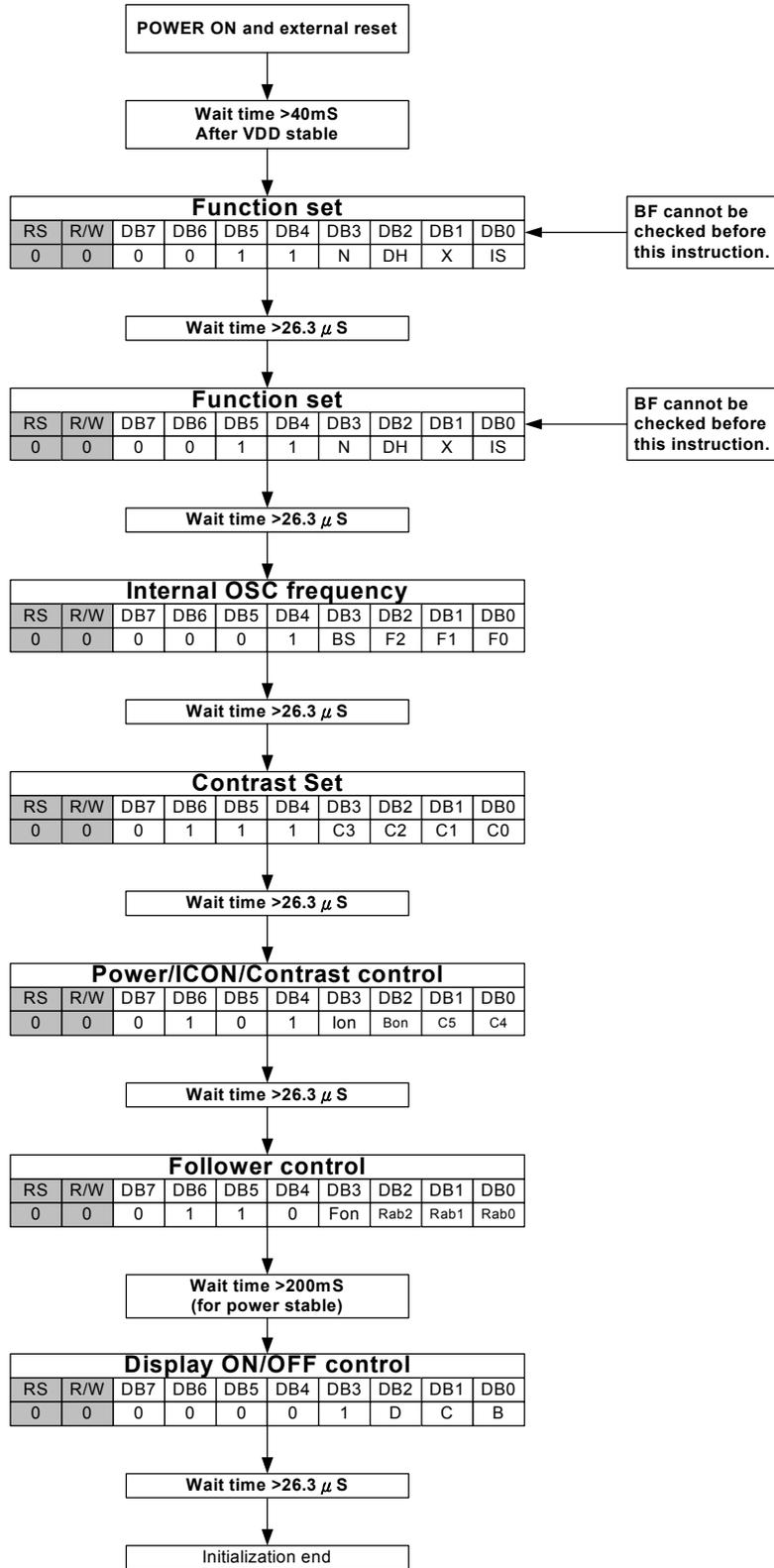
➤ **Initial Program Code Example For 8051 MPU(8 Bit Interface):**
