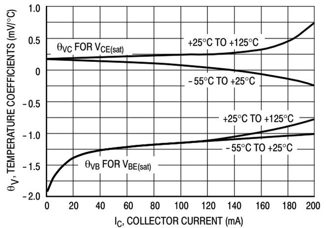
Figure 16. Temperature Coefficients
