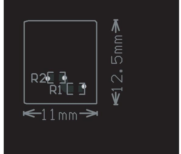
Figure 3: AAT1217 Evaluation Board Layout Example Bottom Layer.
