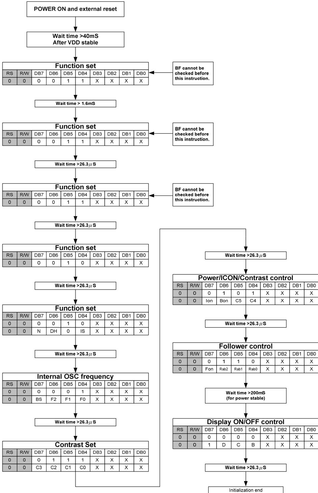
➤ Initial Program Code Example For 8051 MPU(4 Bit Interface):
