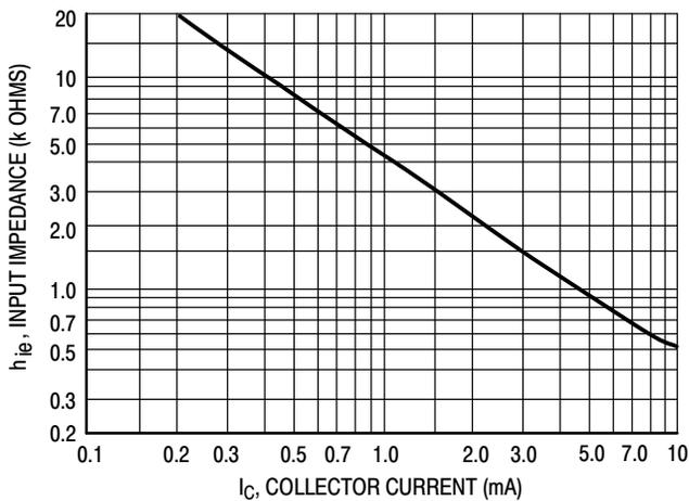
Figure 11. Input Impedance
