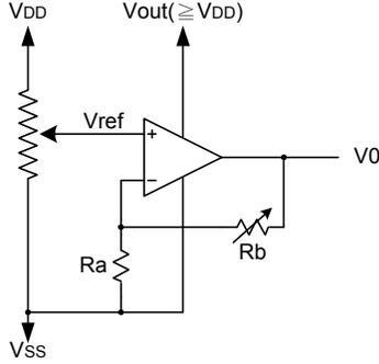
$$V0 = \left(1 + \frac{R_b}{R_a}\right) * V_{ref}$$
